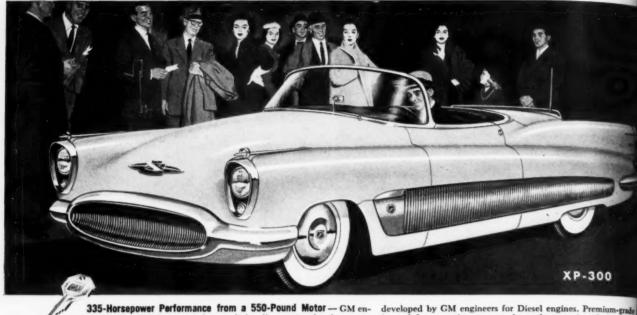
gineers developed an entirely new light alloy engine for these cars. It is a V-8, with 10 to 1 compression ratio, supercharged by a blower
