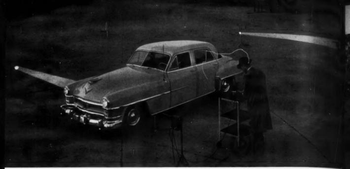
TIMED BY ELECTRIC EYE, Chrysler breaks light beams at start and finish of getaway test, while electronic machines measure
