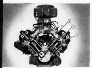
HEART of new De Soto engine. Arrow No. 1 points to dome-shaped combustion chamber. This permits bigger, high-lift valves (No. 2). No. 3 is wide channel for fuel passage. Note absence of sharp bends that slow down "breathing." Like Chrysler Fire-Power, De Soto's Fire Dome loafs at normal speeds but has power reserve that owners really like!
