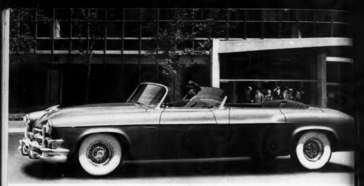
THE NEW PHAETON is a Chrysler-built custom automobile. Powering it is the Chrysler FirePower Engine. It has a wheelbase of 147½" and is distinguished by full-time Power Steering, Oriflow Shock Absorbers, Fluid-Torque Drive and other Chrysler engineering exclusives. Tonneau top is concealed.
