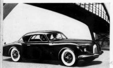
THE K-310, designed and engineered by Chrysler and handcrafted by Ghia of Turin, Italy. Only 59" high, with a wheelbase of 125½", it is designed to use the Chrysler FirePower V8 Engine and full-time Power Steering. This "idea car" represents an entirely new American theme in motor car functional styling.
